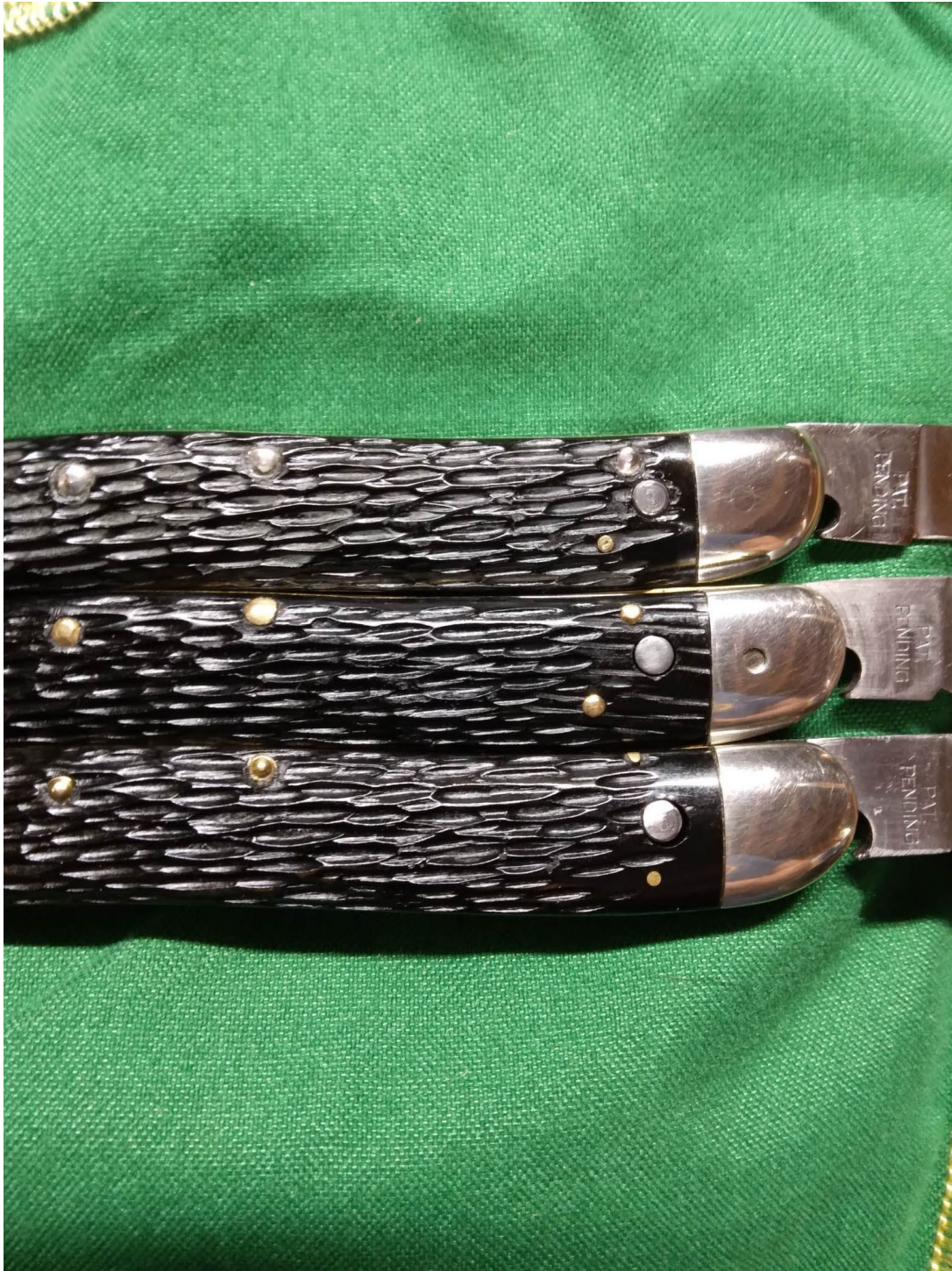
Figure 7. Pile side tang stamps on the same three knives in figure 6, all with "PAT PENDING." We also use images in Figures 6 and 7, to permit direct comparison of center pin differences. The middle knife is clearly a hammered/flat pin as compared to the top and bottom knives where "spinning marks" can easily be seen. The top bolster pin also shows a bit indented. – Thus, the middle knife is a "parts knife" in our opinion (see page 12).
