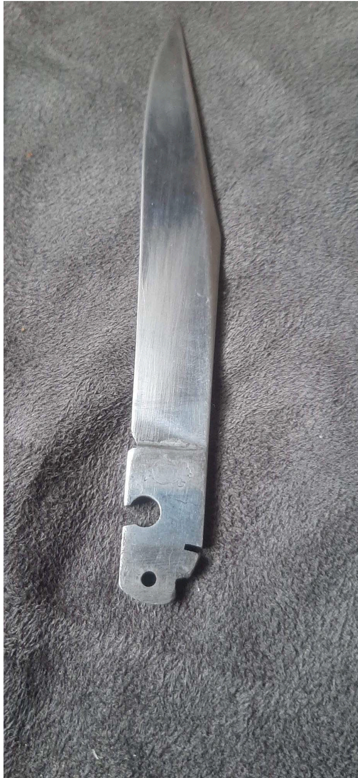
Figure 11. Example of a third modification to make #25 Jet into a lockblade – note the deep notch at the back of the very bottom of the blade, as shown in Figure 10. This blade is a part that was sold from the factory now in a private collection. You can faintly see the "big Q" tang stamp, while the pile side shows the patent number, as in Figure 9. (© Bob Cahill).
