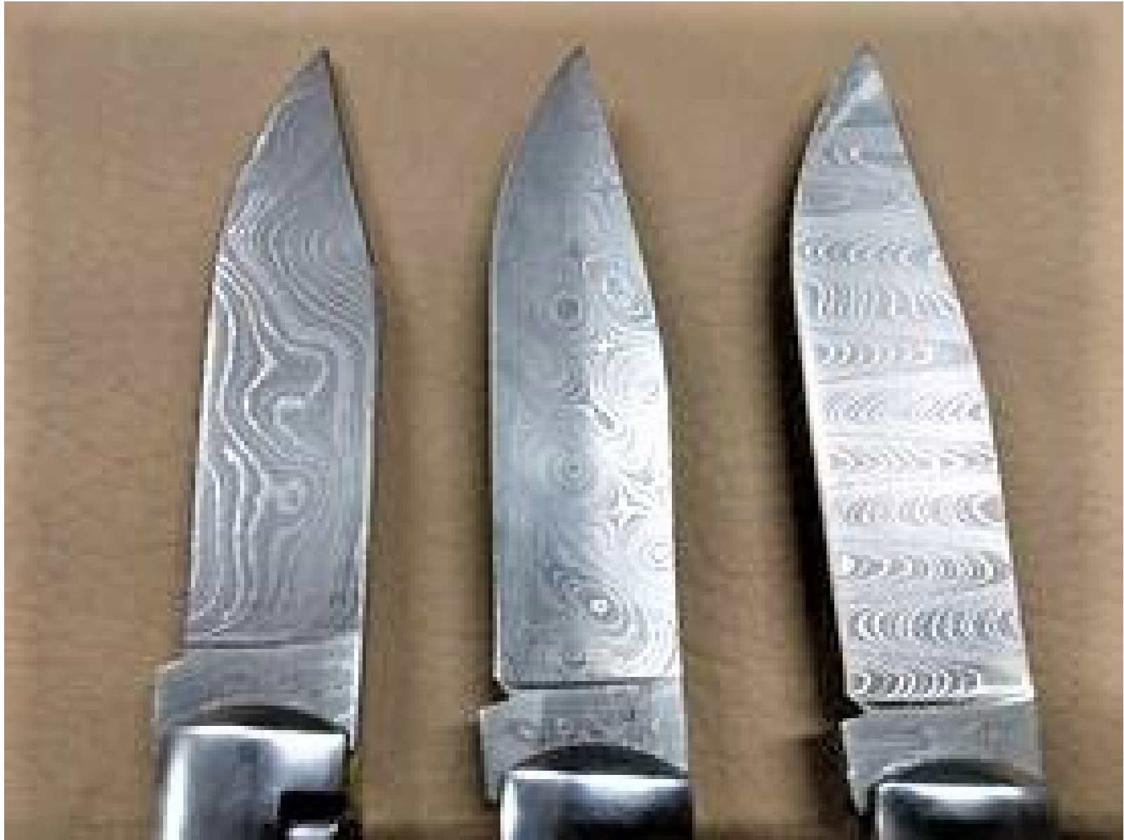
Figure 2. All publicly sold Damascus blades, produced by Alabama Damascus Steel, were in Clip Point style, but three different forms of Damascus patterns were used with each handle material. These are labeled, from Left: Wave pattern, Birdseye pattern, and Ladder Pattern.
