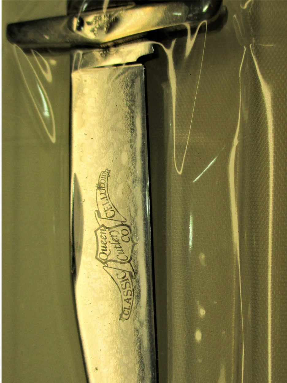
Figure 3. A celluloid etch on the blade of a swing guard knife. While the PH-D2 tang mark on the guard is somewhat hard to see, it is there. This image permits a close look at the blade inside its vacuumed-sealed holder. This experiment was begun 13 years ago, and while you can see some old "oil-bumps" on the blade, so far, the knife shows no damage. So, this article has prompted a review of this plan. Maybe time to clean and re-seal this knife.
