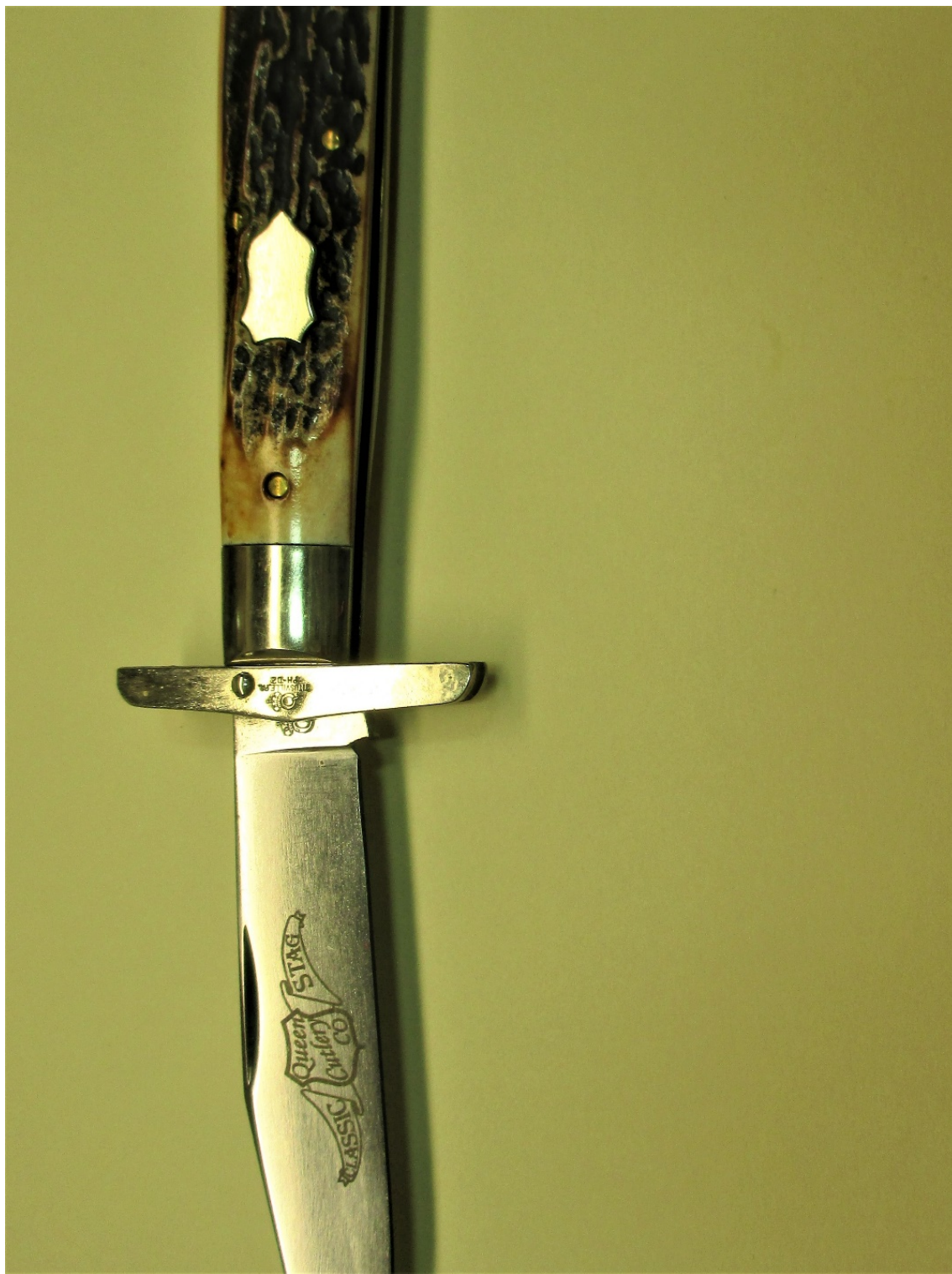
Figure 5. A swing guard in torched Sambar stag with the matching blade etch. The stag on this knife is superb, but the focus in this story is the etches, so no of these images do justice to the attractiveness of the total knives in this series.
