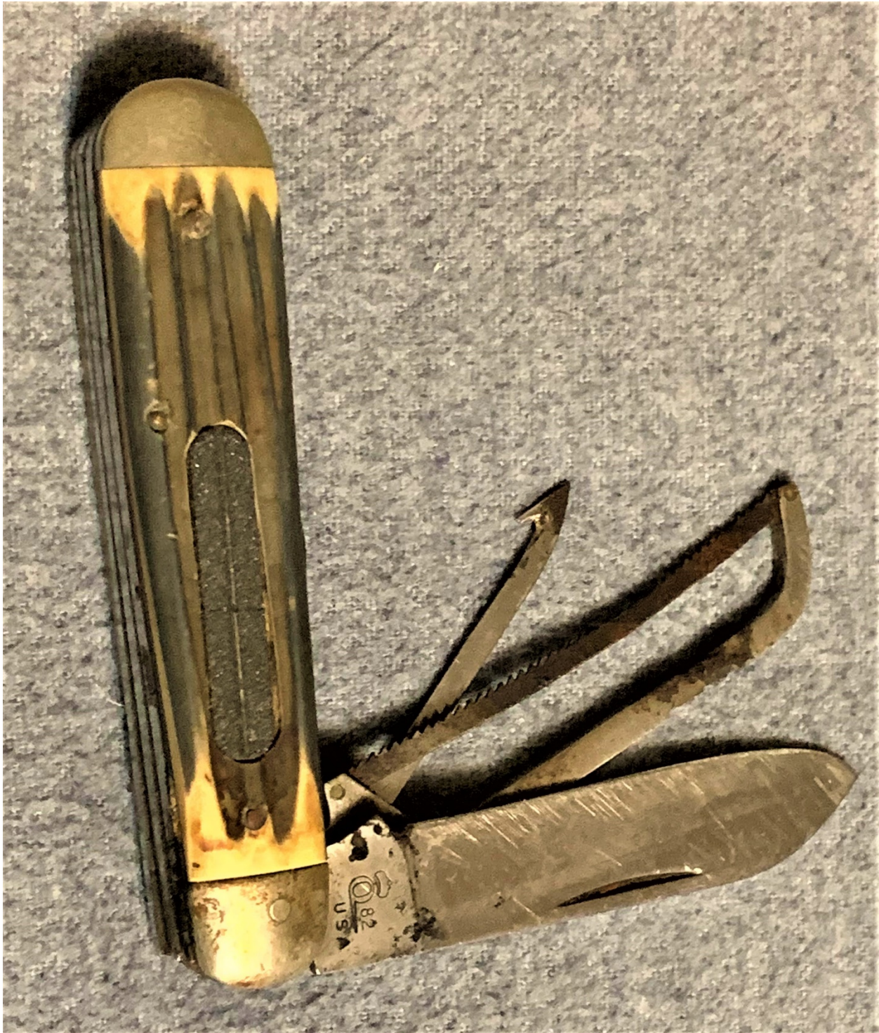
Figure 6. A well-used Joe Z. Rooster, faded delrin, broken whetstone, bent saw, rough sharpening, and tarnish on stainless blades. These knives were not meant for "collectors," and might well characterize the knives a collector might find today.
