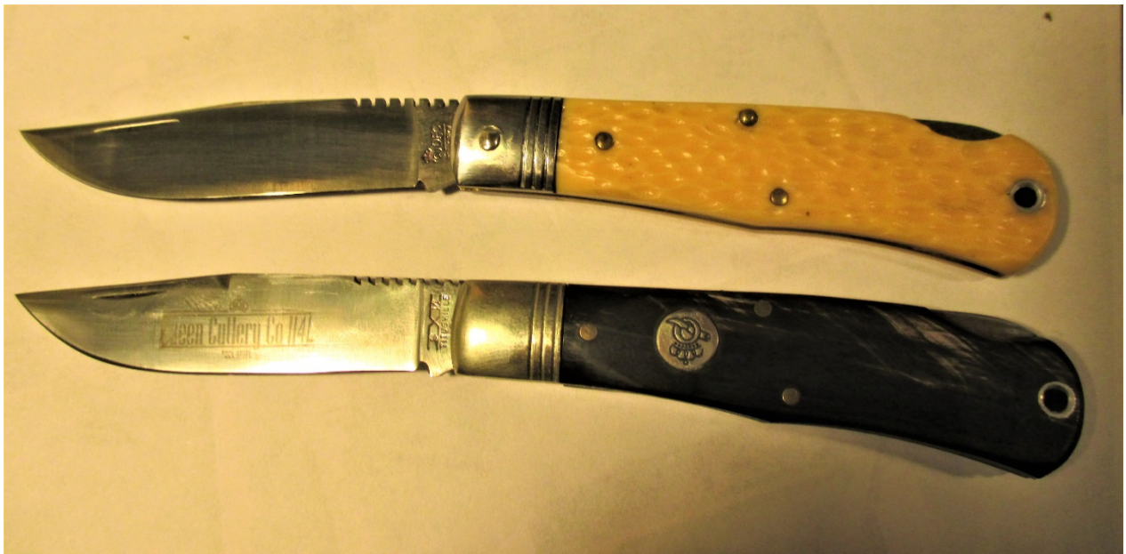
Figure 4. Top, 4L with yellow jiggled delrin handle and very unusual "big pin" style. The bottom knife is smooth feathered Buffalo horn, to show the D2 "tool Steel" etch on the blade -the only cataloged knife with D2.
