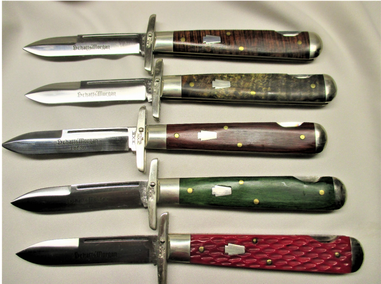
Figure 13. A swing guard series made late in 2016 by the Daniels family with a traditional spear blade with saber grind and long pull, and with Schatt & Morgan keystone shields and blade identifications. From the top the handle materials include a dark brown curly maple, a golden curly maple, Smooth Rosewood, Green smooth wood, and red jugged bone. Each of these knives was produced in very limited numbers that are not labeled on the blade. Some were claimed to be 1 of 1 (red jugged bone) others up to 10 (smooth rosewood). There may well be other similar knives that disappeared into collections before they could be documented.
