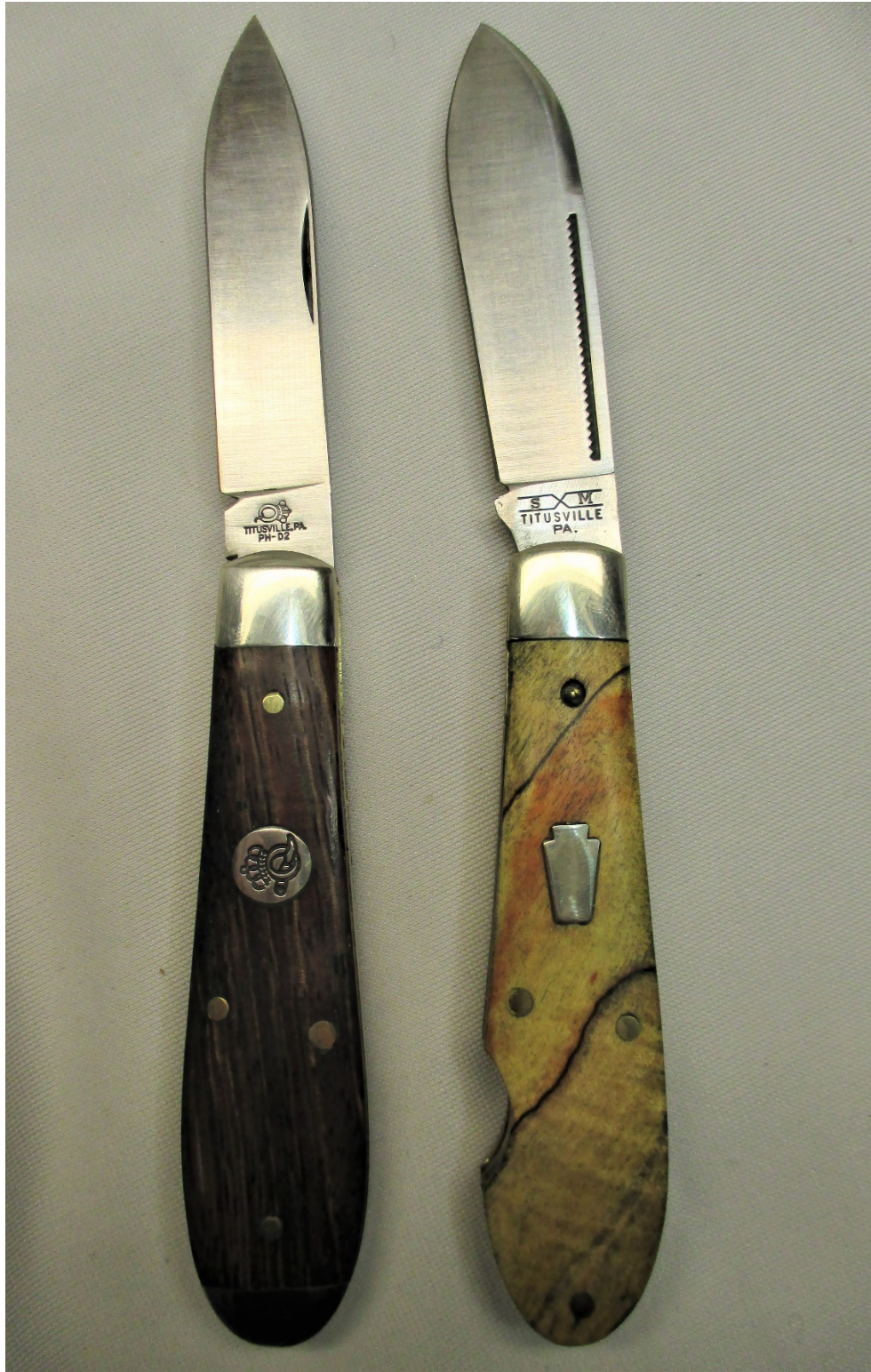
Figure 6. two single blade #06. On left is very late production, with D2 steel, but using "incised" rather than "relief" shield, and coarser wood of unknown type (no "tool steel" etch.) On right is an "easy open" version with probably a stabilized maple wood and satin finish large spear blade with no etch. Again, more roughness around the keystone shield.
